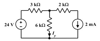
a. How many equations are necessary to analyze this circuit by the mesh analysis method?
